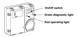
On OEM installs the 'red" & "green" indicator lights illuminate. On after market installs only the "Red" light illuminates.
