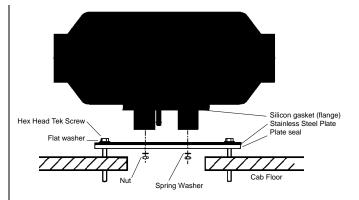
Note: Tighten screws sufficiently to ensure positive seal between mounting plate and mounting surface.
